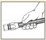
Step 7. Important—Check hose for pushout by observing hose position mark. Pushout should not be evident. CLEAN, PROOF TEST TO TWICE OPERATING PRESSURE AND INSPECT ALL ASSEMBLIES. Disassemble in reverse order.
