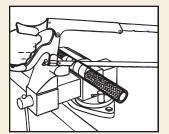
Step 1. Cut hose square to length with fine-tooth hack saw or cut-off wheel. To minimize wire braid flare out, wrap hose with masking tape and cut through tape. Remove tape before next step.
