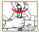
Step 5. Carefully insert nipple and engage nipple and socket threads while holding hose in position with other hand. Make sure hose does not push out of socket by observing mark made in Step 3.
