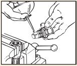
Step 4. Lubricate inside of hose and nipple threads liberally using S.A.E. 30 lubricating oil.
