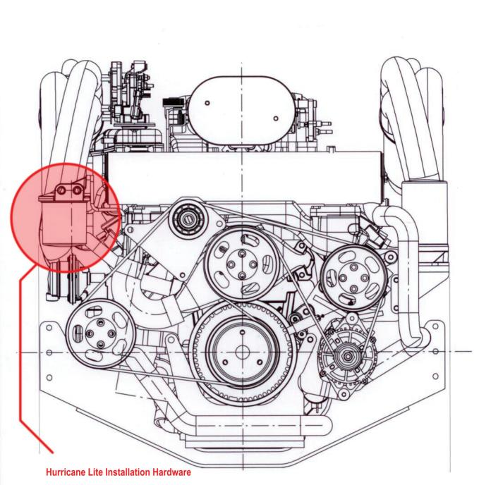
(1) Fuel Filter relocation bracket allows filter assembly to be moved slightly forward to accommodate larger outer "Cooling" exhaust tube of the Hurricane Lite headers. (4) 5/16 x1-1/2" bolts and nuts are supplied for reattaching the fuel water separator and (4) 1/4 X 1" bolts and nuts are supplied for reattachment of the bracket to the engine. There is a 1/4 hole at the end of the bracket that will allow the factory dipstick mounting tab to be straightened out and attached to this location.
