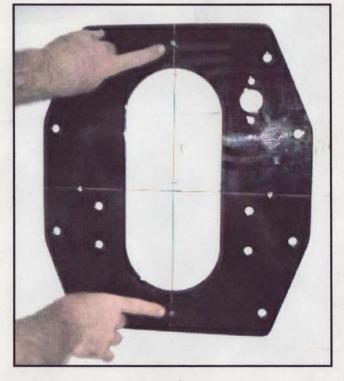
Figure 2: Locating X-dimension Insert dowel pins...
