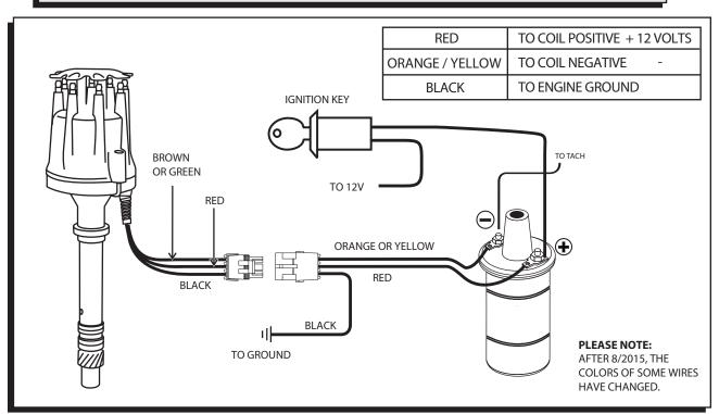
Wiring the Marine Ready-to-Run Distributor.
