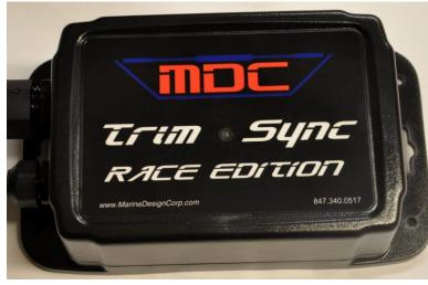
TrimSync monitors the trim for twin and triple engine boats, so when the operator presses the BOTH/ALL button, it will automatically adjust the drives / outboards to be in perfect alignment, every time. You will never have to worry about how accurate your mechanical trim indicators are because TrimSync will always move the slowest drive / outboard to match the others. TrimSync is compatible with all LED and electronic trim indicators. In
