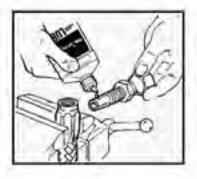
MALE ENDS: Push assembly tool into nipple.
