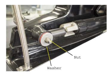
Install trim pin cup on trim pin and secure with nut. Tighten nut until approximately 2 threads are exposed through nut. Do not over tighten nut, as rubber bushings may be damaged.
