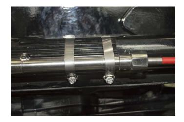
Remove pin from actuator. Cycle actuator several times and watch the actuator for smooth operation
