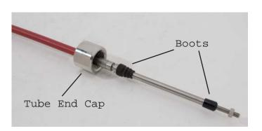
Install cable clip into cable groove. Slide tube end cap over cable clip and secure to the cable with tape.
