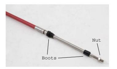
Slide tube end cap onto the cable with threaded opening facing the end of the cable. Replace rubber boots and cable nut.
