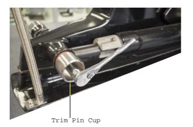
3. Place actuator tube bracket and clamps loosely on the trim ram.
