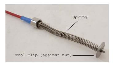
Thread push rod onto the cable end until it contacts the cable nut. Remove tool clip so spring contacts push rod.
