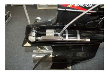
10. If replacing an existing cable system you can remove the cable from the thru hull and use the new center section in the old stainless housing.
