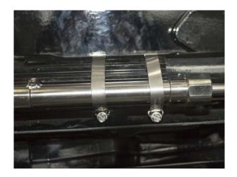
Remove pin from actuator. Cycle actuator several times and watch the actuator for smooth operation
