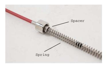
6. Compress spring and install tool clip between spring and cable nut. Slowly release tension on spring until it holds tool clip in place.
