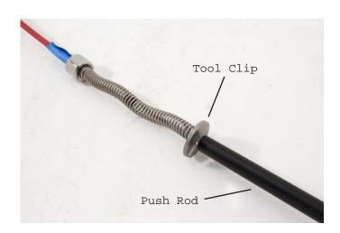
8. Apply liberal coating of an anti-corrosion grease to spring. Install the actuator tube over push rod assembly. Apply a small amount of Loctite 271 to threads of actuator tube.
