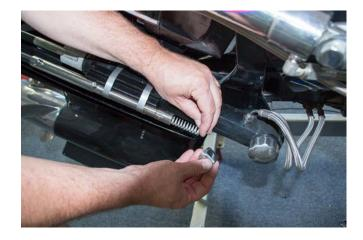
Install the sensor onto the actuator using the two 10/32 screws provided with the cable towards the back of the boat.
