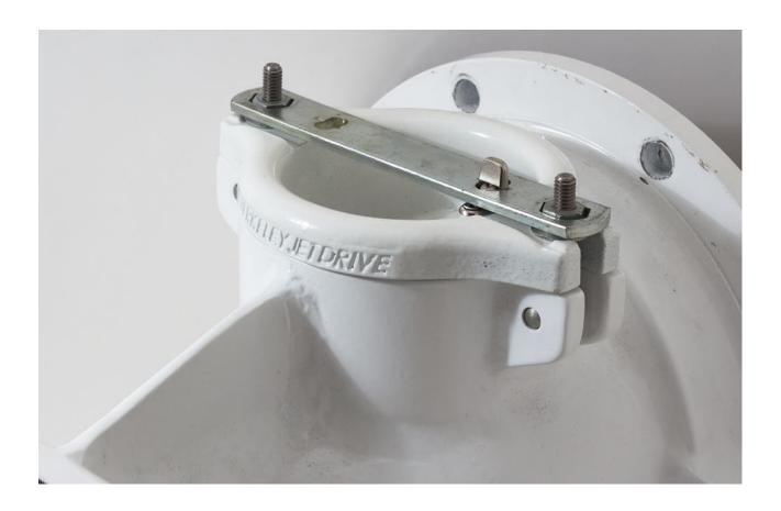
Once the cover fits to your liking tighten the fasteners that retain the cover and install the lock wrench (fig5).
