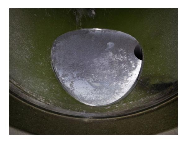
Due to some variations in castings you may have to match the cover to the radius of your pump. This can be done by grinding the cover to match the pump radius, this will give you a nice clean flow of water(fig4).
