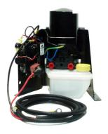
This system is ready to plug into a Mercruiser Wire Harness
