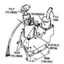
PT470N, PT471NMK, PT475TN-4 & PT476NMK-3 FIT ON THIS DESIGN 1, 3-RAM, INTEGRAL MERCURY T/T SYSTEM WITH SIDE OIL FILL.
