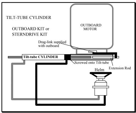
1) Simply fit the extension rod to the piston rod, and secure using a small quantity of loc-tite (1-2 drops only). Make sure the threads are clean and oil-free. This is to prevent the rod from unscrewing once installed. Spanner flats are provided on the piston rod for this purpose. DO NOT GRIP THE PISTON ROD AT ANY TIME WITH ANY TOOLS ON THE WORKING SURFACE OF THE ROD.
