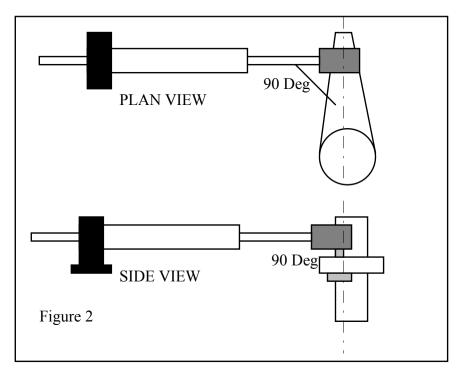
A typical single rudder installation is shown in Fig.2 above. The rudder should be in-line with the tiller arm, and the slave cylinder should be mounted squarely to the tiller arm. Please also note that the cylinder should be both square and parallel to the tiller arm.
