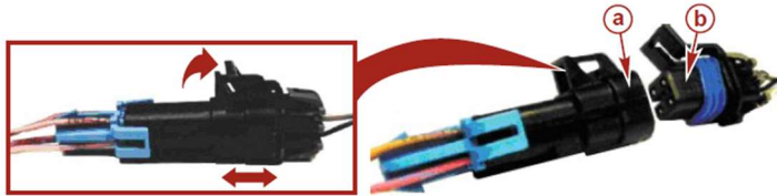
Figure 10 - Four wire oxygen sensor connector, "a" is the engine harness connector and "b" is the sensor connector
