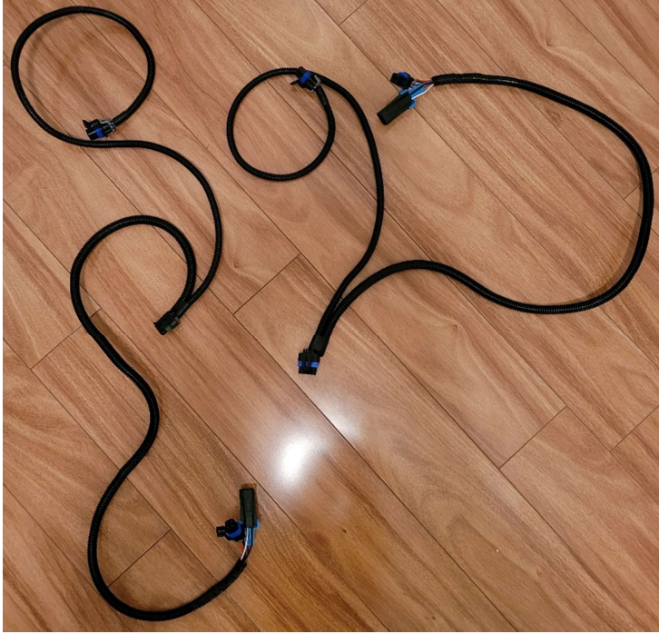
Figure 7 - Each harness of the CEC Kit must feed one engine bank
