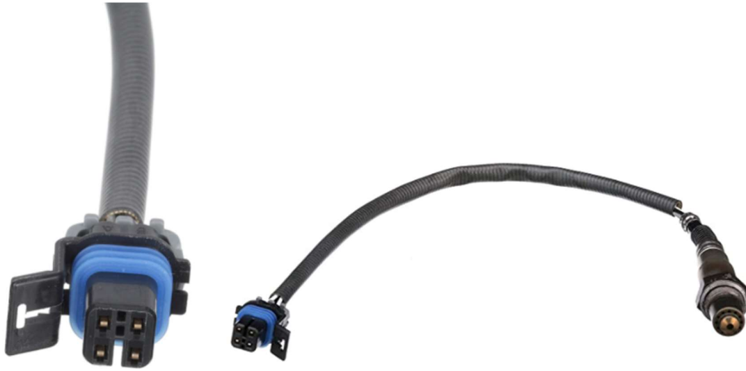
Figure 1 - Four wire oxygen sensor and connector
