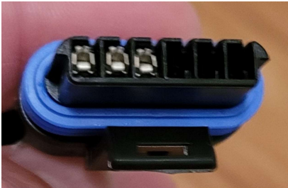
Figure 11 - The six pin connector uses only three pins
