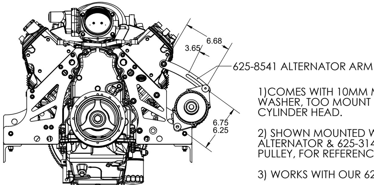
1) COMES WITH 10MM MOUNTING BOLT & WASHER, TOO MOUNT FLAT AGAINST THE CYLINDER HEAD.
